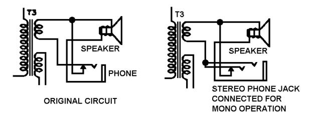
However, you MUST use ONLY a STEREO mini phone plug in the new headphone jack. There are mono mini plugs and, if you insert a mono mini plug into the stereo jack (as wired in the above diagram) the ring connection in the jack will short to the sleeve. This is because the mono plug has no ring. This won't cause any harm but will short out the signal and you won't hear anything.
